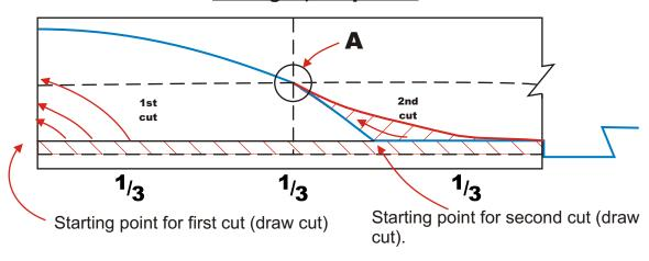
Blend second cut into first cut at point A.
